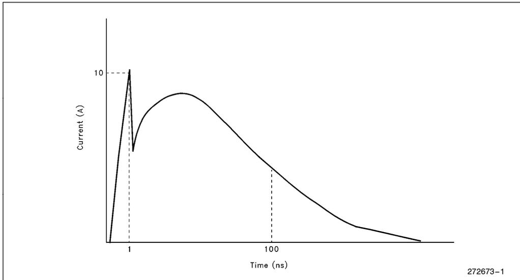
Figure 1. Typical Waveshape of ESD from Human Body
