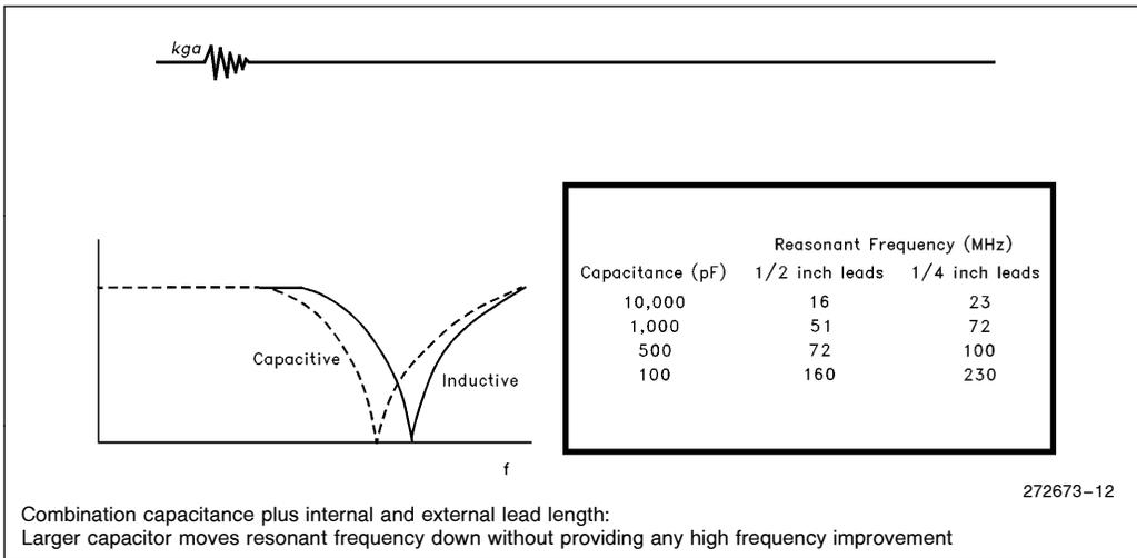
**Figure 13. Capacitor Resonance**
