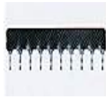
Single In-Line Package ("SIP") in 4 pin to 13 pin package
