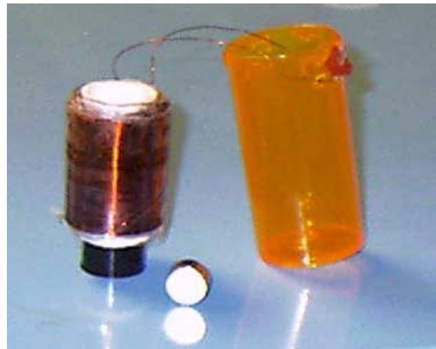
Figure 4: The finished solenoid with cylindrically symmetric magnet and prescription pill container.
