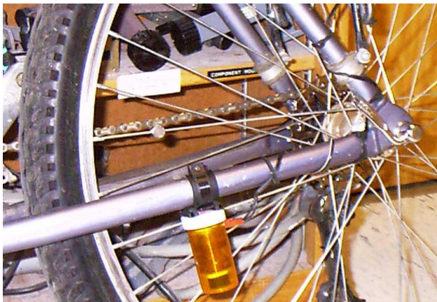
Figure 5: Completed version of the generating part of the device.
