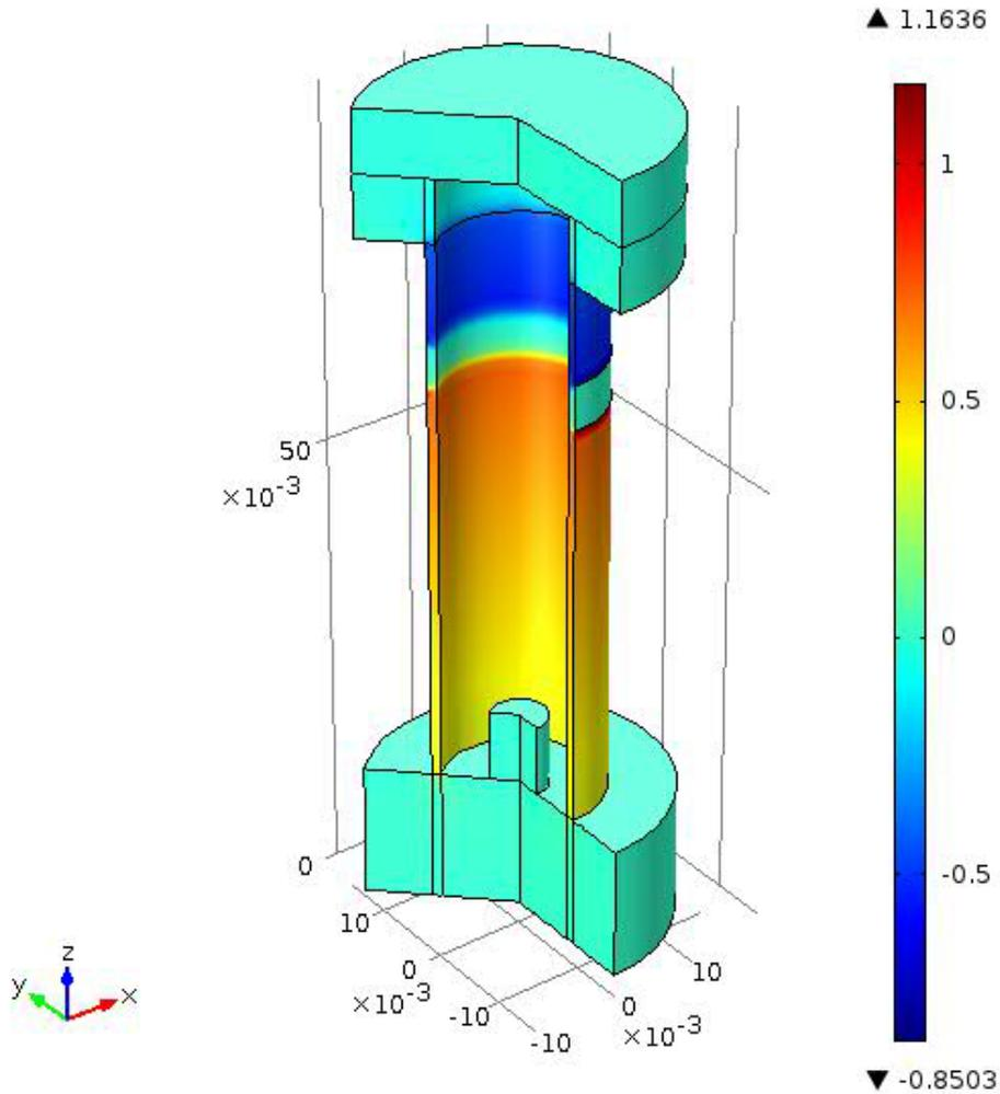
**Figure 4.** COMSOL simulation of the temperature gradient in the stainless steel vessel as a result of the local heating around the neck of the vessel. In this particular notation the temperature gradient is positive towards the bottom of the vessel. The portion of the vessel above the heating rings conducts heat as well, but the gradient is in the opposite direction, represented by the negative value.
