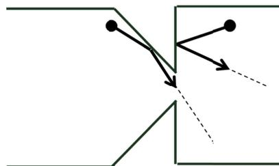
Figure 5. Top view of charge carriers reflecting off the edges of a geometric diode.
