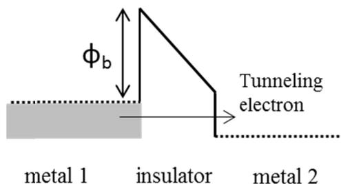
Figure 3. A typical band diagram of a metal-insulator-metal diode under applied bias. The Fermi levels of the two metal layers and the conduction band edge of the insulator are shown as function of position. In this diode, the barrier height at metal 1 is the energy amount of  $\Phi_b$  and is larger than that at metal 2. Electrons tunnel from metal 1 to metal 2 through the insulator.
