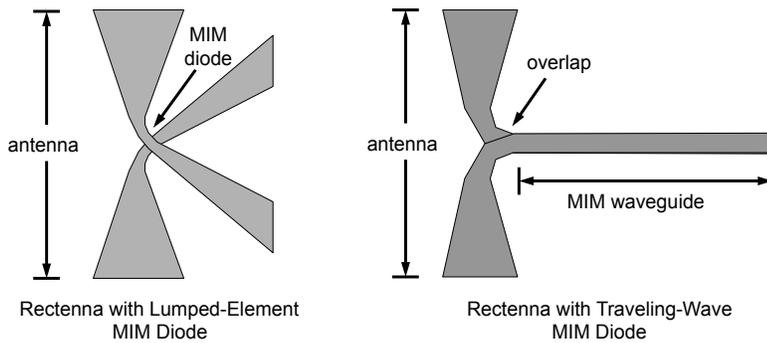
Figure 4. Comparison of lumped-element and traveling-wave MIM diodes in a rectenna (top view).
