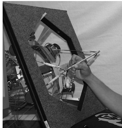
Fig. 1. Parallel haptic interface with 5 prismatic actuators connected to a hand-held stylus.
