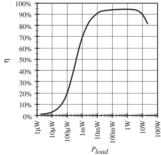
Fig. 11. Predicted converter efficiency vs. output power, variable frequency converter.
