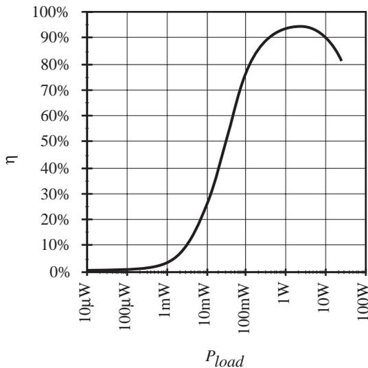
Fig. 6. Predicted converter efficiency vs. output power, conventional fixed frequency converter.
