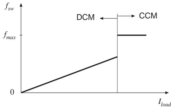
Fig. 10. The operating range can be further extended by use of the continuous conduction mode near full load, and variable frequency discontinuous conduction mode at light load.
