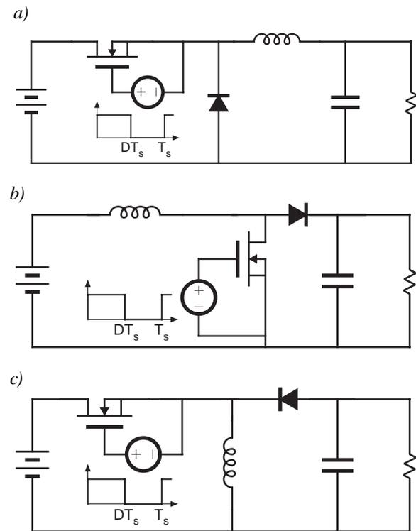
Fig. 3. Basic dc-dc switching converter circuits: (a) buck, (b) boost, (c) buck-boost.
