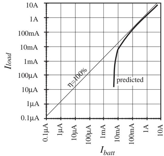
Fig. 7. Predicted converter input current vs. output current, conventional fixed frequency converter.
