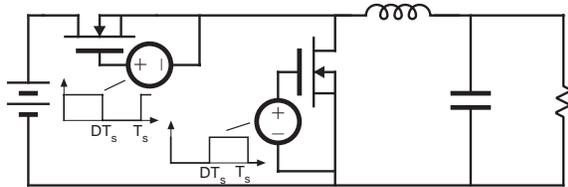
Fig. 5. Buck converter with synchronous rectification.
