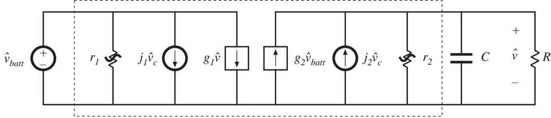
Fig. 14. Equivalent circuit model which predicts the small-signal transfer functions of variable-frequency DCM converters.
