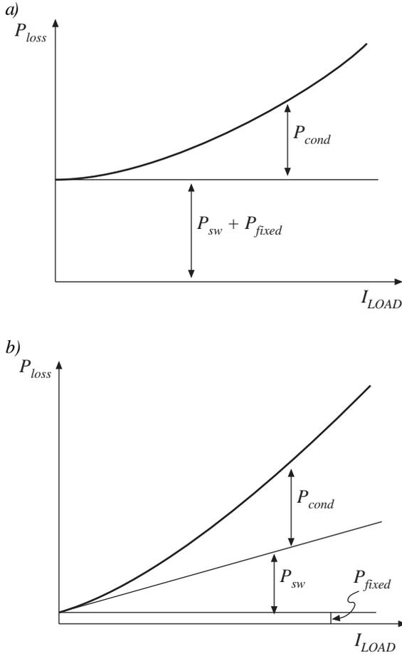
Fig. 2. Variation of converter power losses with load current: (a) in a conventional fixed-frequency converter; (b) with switching frequency proportional to load current.
