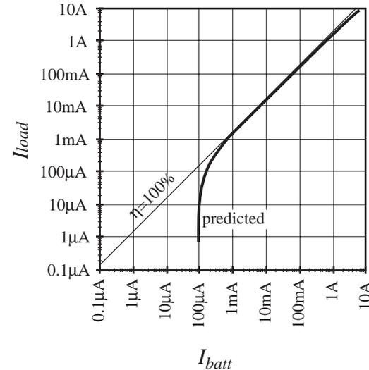
Fig. 12. Predicted converter input current vs. output current, variable frequency converter.
