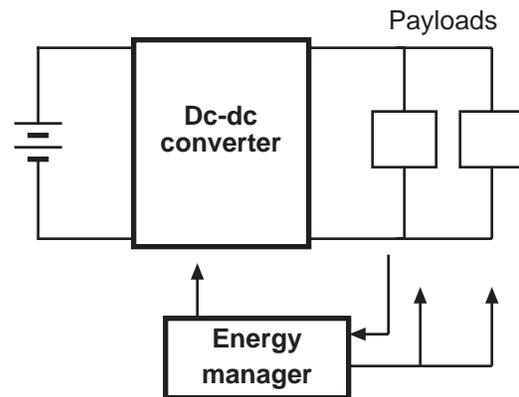
Fig. 1. A simple energy management system for a battery-powered mobile system.
