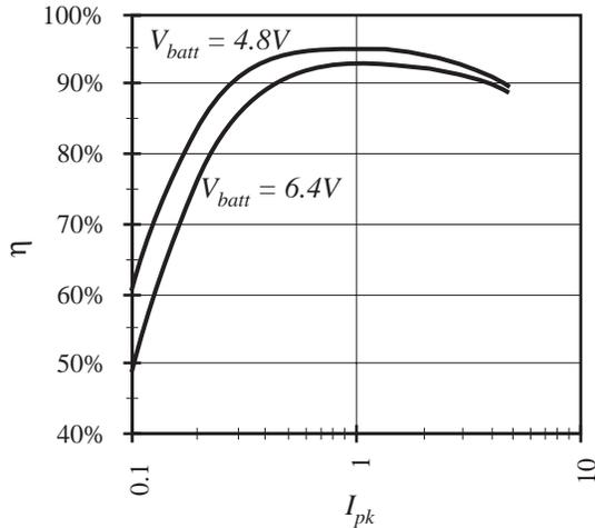
Fig. 9. Efficiency vs. peak transistor current, for constant-current-programmed DCM buck converter example with variable-frequency control
