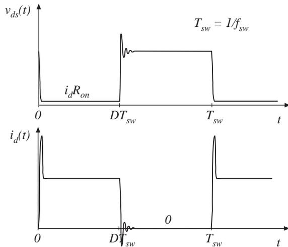
Fig. 4. Typical MOSFET voltage and current waveforms in a conventional dc-dc converter operating in continuous conduction mode.
