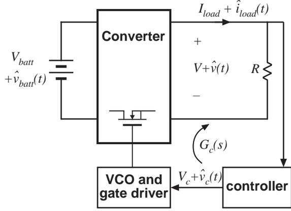
Fig. 13. Output voltage regulation system block diagram.
