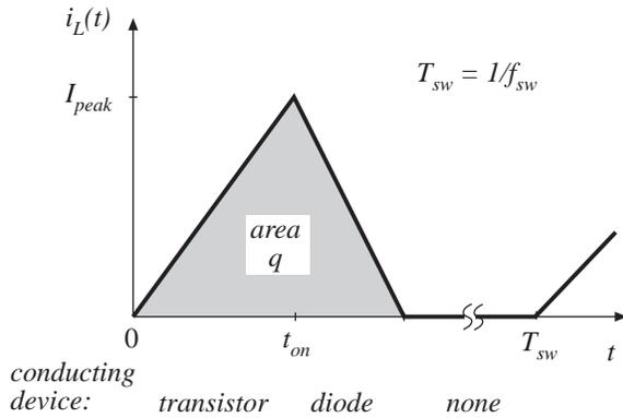
Fig. 8. Inductor current waveform  $i_L(t)$  in the discontinuous conduction mode.
