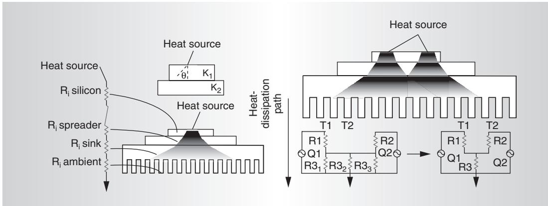
Figure 1. Thermal modeling of an on-chip router. Modeling is based on the idea of heat-spreading angle, which lets designers accurately characterize the package's heat-dissipation path.
