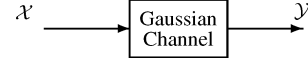
Fig. 2. The Gaussian channel. If the set \mathcal{X} contains jointly Gaussian variables, then the set \{\mathcal{X}, \mathcal{Y}\} is jointly Gaussian.
