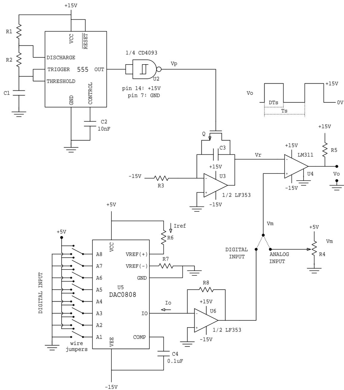
Figure 4: Complete circuit of the pulse width modulator.
