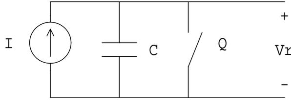
Figure 2: A conceptual saw-tooth generator.
