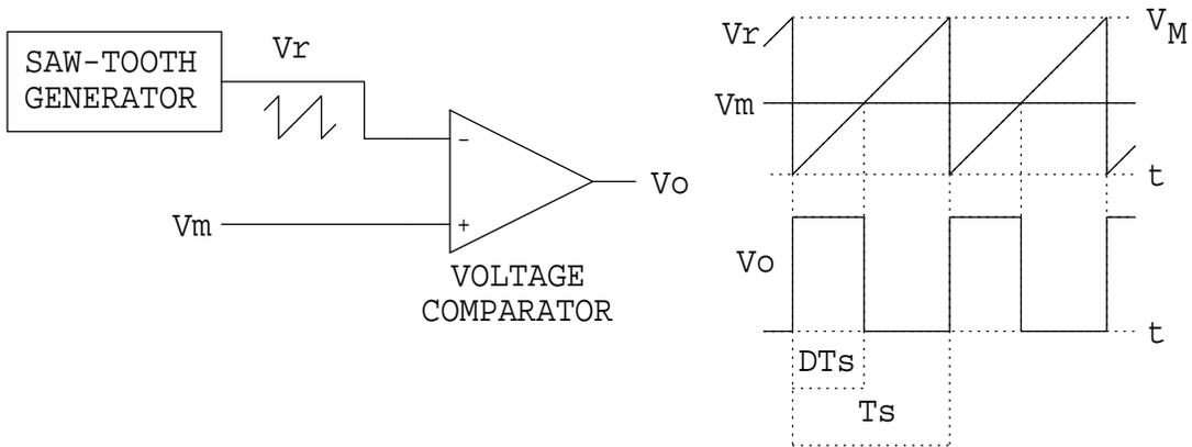
Figure 1: Pulse width modulation using a saw-tooth generator and a voltage comparator.
