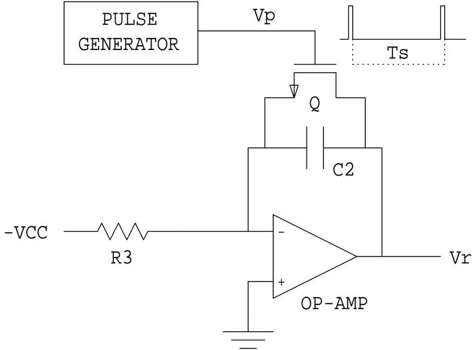
Figure 3: A saw-tooth generator using a pulse generator and an op-amp integrator with reset.
